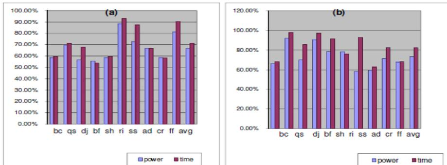
Figure. 6. Percentage of power and access time reduction with prefetching for (a) instruction and (b) data caches
