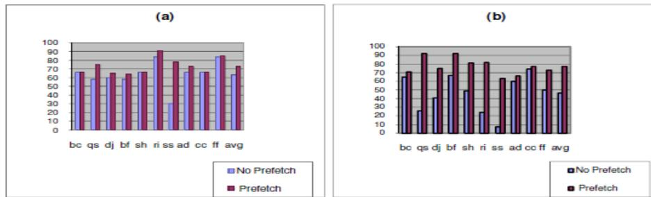
Figure. 9. Percentage of dynamic and static power reduction without and with prefetching for (a) instruction and (b) data caches
