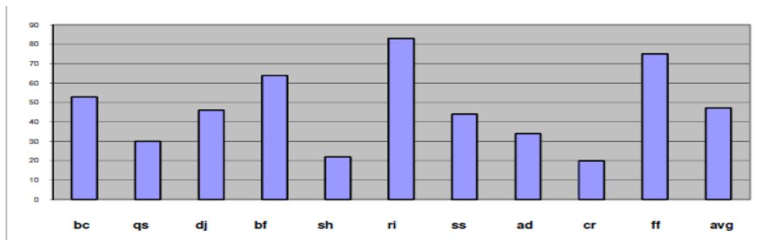
Figure. 8. Percentage reduction of execution cycle after implementing branch prediction
