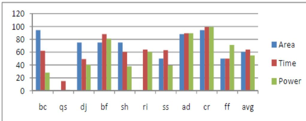
Figure 4(b). Percentage reduction of area, power and cache access time for L-2 data caches
